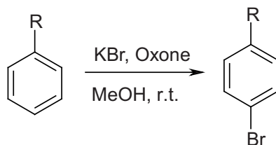
Figure 3: Bromination on aromatic compound using potassium peroxymonosulfate
